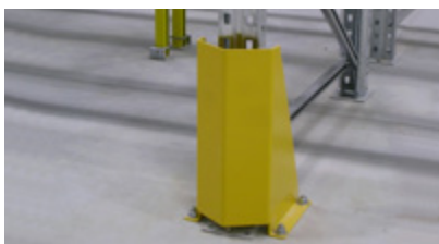
Floor mounted Column Guard Protection for pallet racking uprights.
